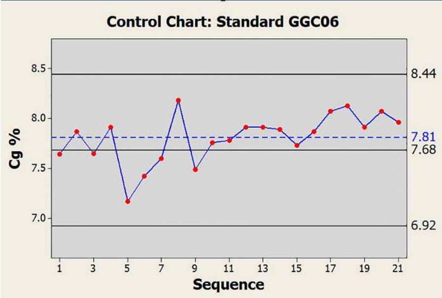
\*\* Expected value = 7.68% graphitic carbon; sample mean = 7.81% graphitic carbon
