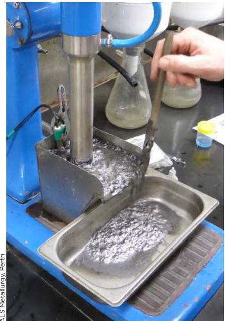
Figure 9: Graphite flotation test
