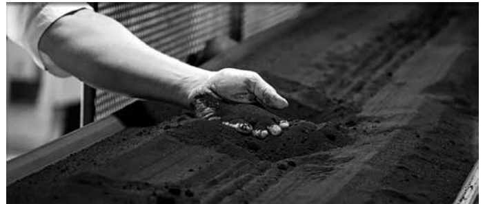
Figure 3. Moulding sand used for metal-casting applications. Known as “greensand” this incorporates silica sand, bentonite and carbonaceous additives. Bentonite is the bonding agent and is typically qualified according to mechanical properties such as green, dry and wet tensile strengths, in addition to thermal durability. Source: AMCOL Metalcasting.
