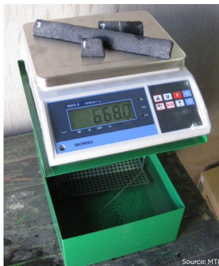
Figure 1. Archimedes (water displacement) equipment. Chromitite sample being weighed in air.
