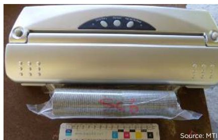
Figure 4. Vacuum-packing a pyroxenite core sample.
