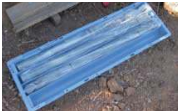
Bentonite core sealed inside plastic to preserve in situ moisture content. Source: MTI
