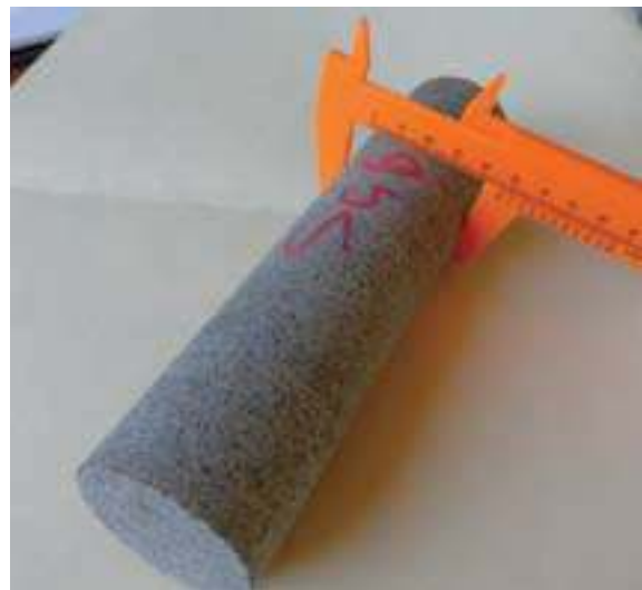
Pyroxenite core sample being measured using a calliper. Source: MTI
