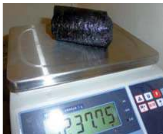
2 Paraffin wax coated friable chromitite sample being weighed in air. Source: MTI
