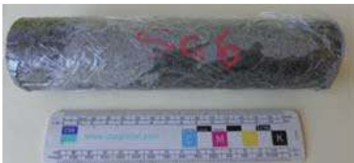
Pyroxenite core covered with cling wrap, illustrating water ingress. Source: MTI
