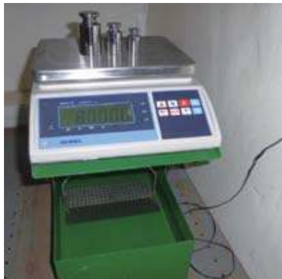
Calibration of a density balance using standard weights. Source: MTI
