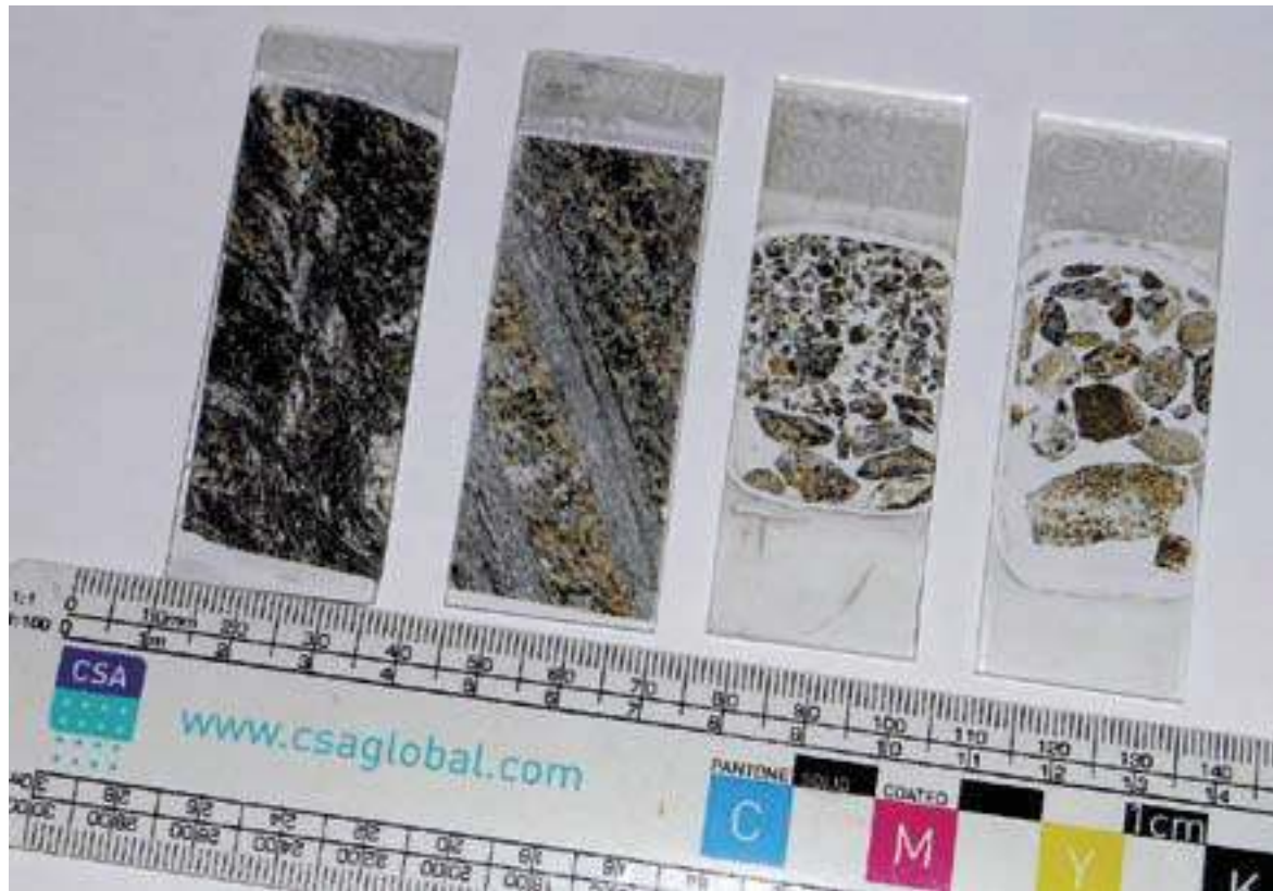
Polished thin sections made from core or outcrop (two samples on the left) and RC chips (two samples on the right)
