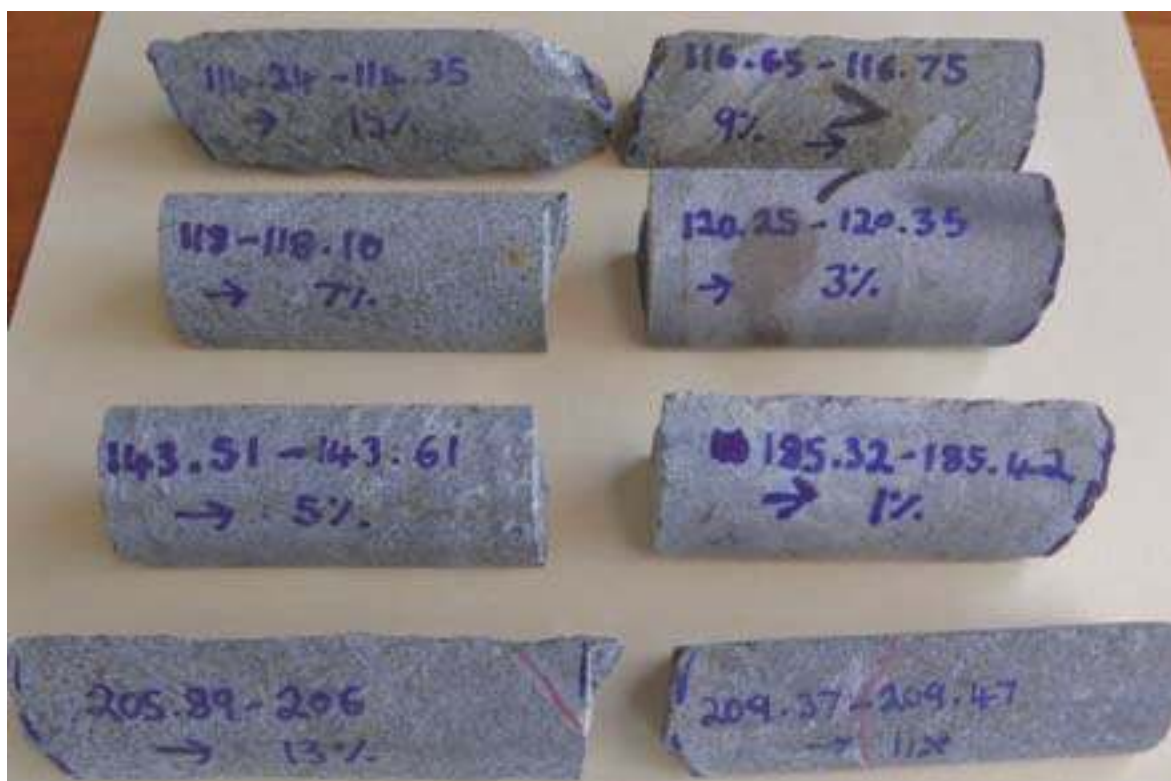
Core samples representative of rock types on a specific project. Approximate graphite contents indicated as percentages.
