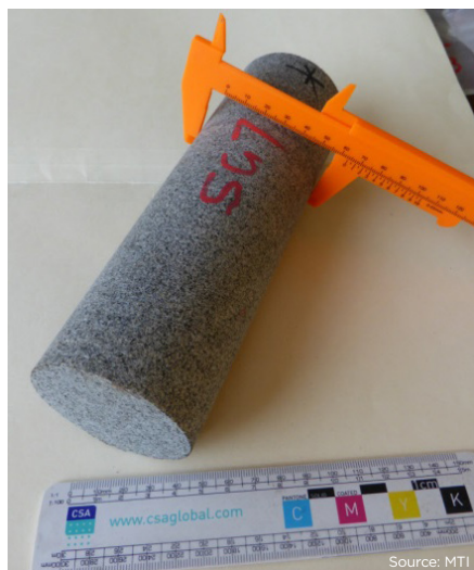
Figure 5. Pyroxenite core sample being measured using a calliper.
