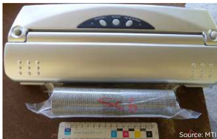
Figure 4. Vacuum-packing a pyroxenite core sample.
