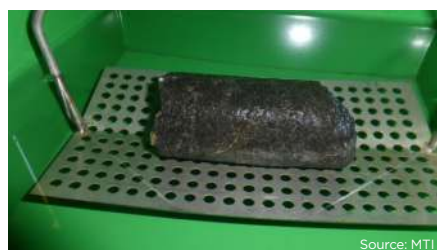
Figure 2. Wax-coated friable chromitite core sample being weighed in water.
