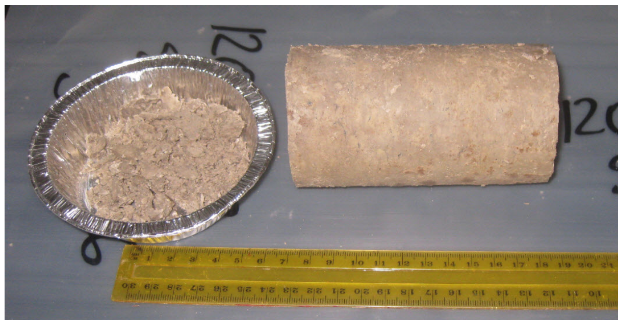
Figure 4. Bentonite core trimmed for calliper method. The core 'shavings' were used for moisture analysis.
