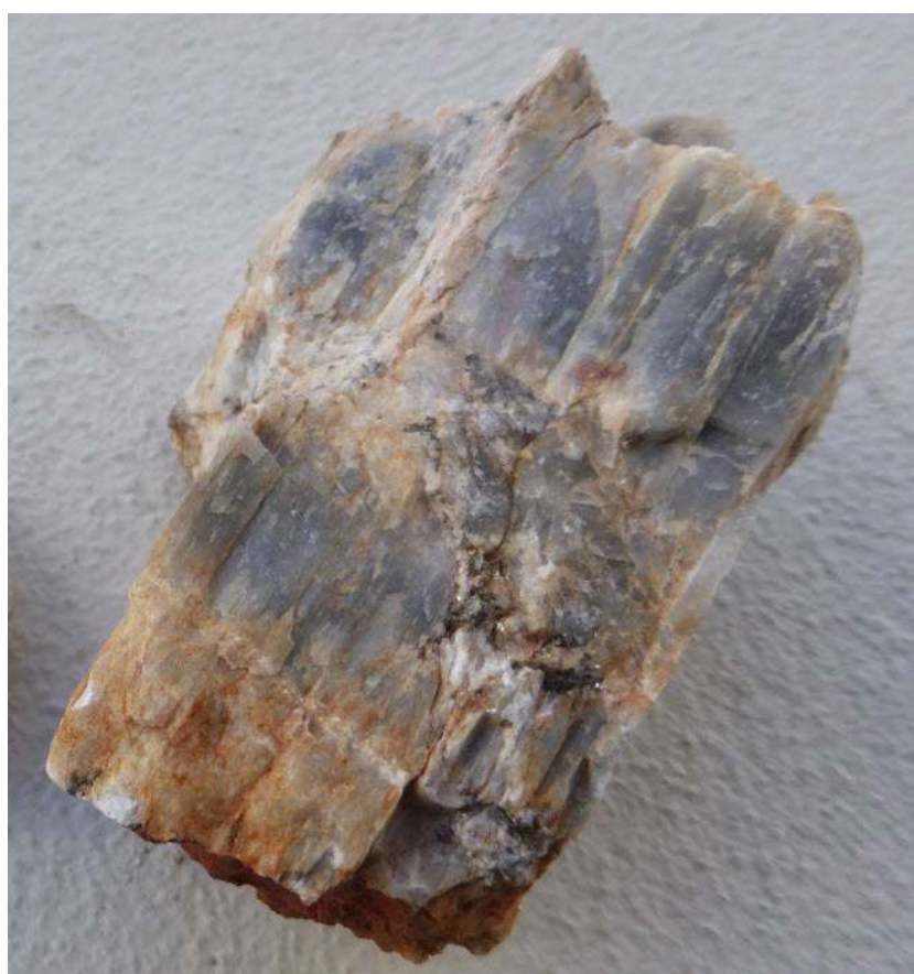
Figure 1. Hand specimen of petalite, spodumene, feldspar and quartz with minor mica, from a pegmatite outcrop. Sample length approximately 15cm
