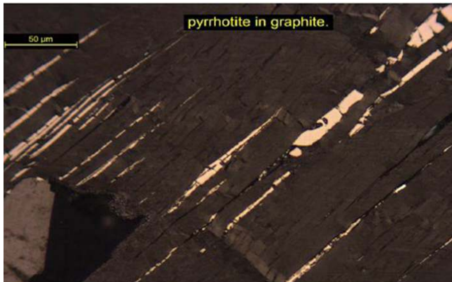
Figure 6: Photomicrograph illustrating pyrrhotite interleafed with graphite. Scale bar = 50 micron.
